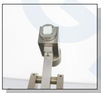
This tester put the dry and wet felted wool on the friction mallet surface, rub the specimen move back and forth in a certain process and speed on the friction table for a certain times, and then evaluate its damage and decoloring degree.
